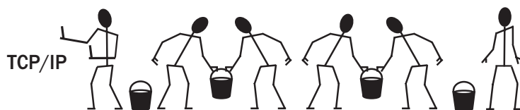
TCP/IP is receiver controlled, like a bucket brigade. The size of the buckets and the rate at which they are transferred can be varied by the receiver.
